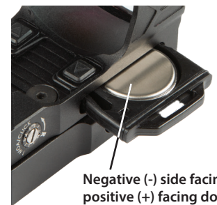
1* - Battery Compartment Detail
