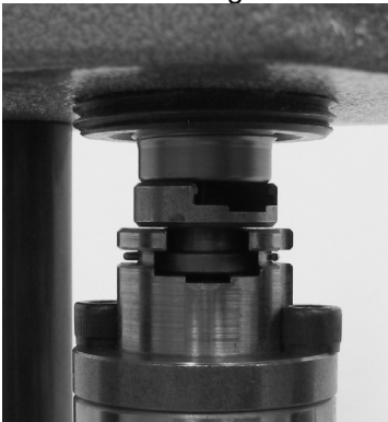
Photo 4 - Size die to shell holder contact
