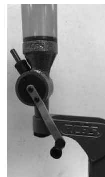
Dispensing Metered Charge (Handle Down)
