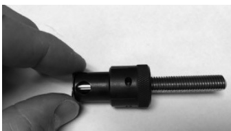
Metering Screw threaded into Bushing
